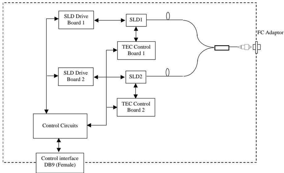
Figure 1 Configuration of IPSDW0825-xxxxx SLD light source module
