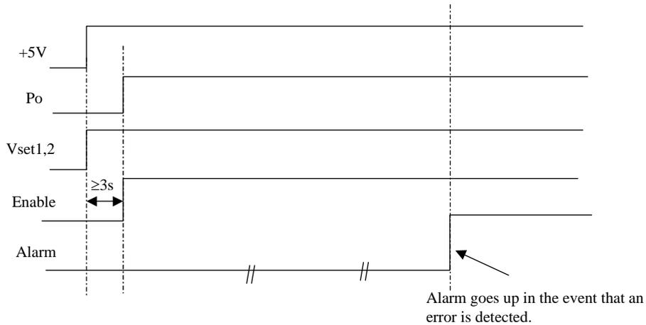
Figure 3 Startup and operational timing of IPSDW0825 module
